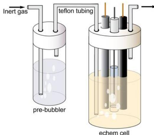
not perturbing the solution in the cell. Another option is to feed electrode cables into an inert atmosphere glovebox and run electrochemical experiments using previously deoxygenated solvents.
