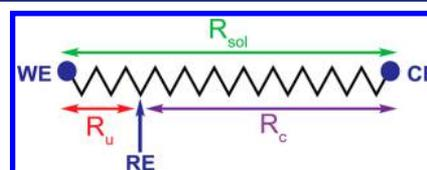
**Figure 5.** Representation of an electrochemical cell as a potentiostat. Adapted from ref 1. Copyright © 2006, with permission from Elsevier. Increasing the conductivity of the solution diminishes  $R_{\text{sol}}$  and, therefore,  $R_u$ . Diminishing the distance between WE and RE diminishes  $R_u$ .  $R_c$  is generally compensated by the potentiostat.
