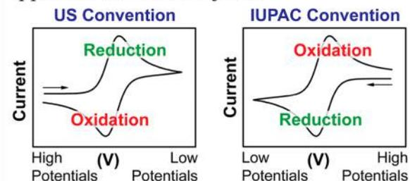
direction in which the potential was scanned to record the data. The arrow indicates the beginning and sweep direction of the first segment (or “forward scan”), and the caption indicates the conditions of the experiment. A crucial parameter can be found in the caption of Figure 2: “ $v = 100$  mV/s”. This value is called the scan rate ( $v$ ). It indicates that during the experiment the potential was varied linearly at the speed (scan rate) of 100 mV per second.
