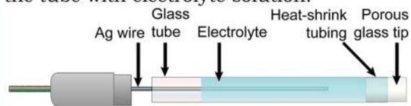
presumably takes advantage of the natural oxide layer on the silver wire, using the resulting ill-defined Ag<sub>2</sub>O/Ag couple. This method eliminates the possibility of silver salts leaks but requires the presence of an internal standard.
