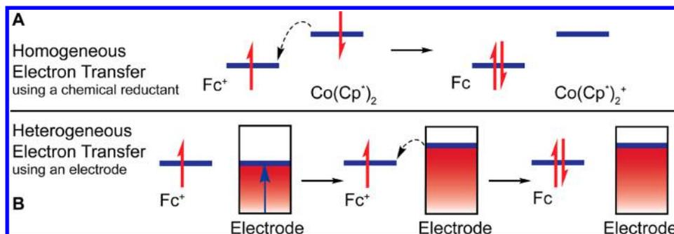
**Figure 1.** (A) Homogeneous and (B) heterogeneous reduction of  $\text{Fc}^+$  to  $\text{Fc}$ . The energy of the electrons in the electrode is controlled by the potentiostat; their energy can be increased until electron transfer becomes favorable.<sup>4</sup>
